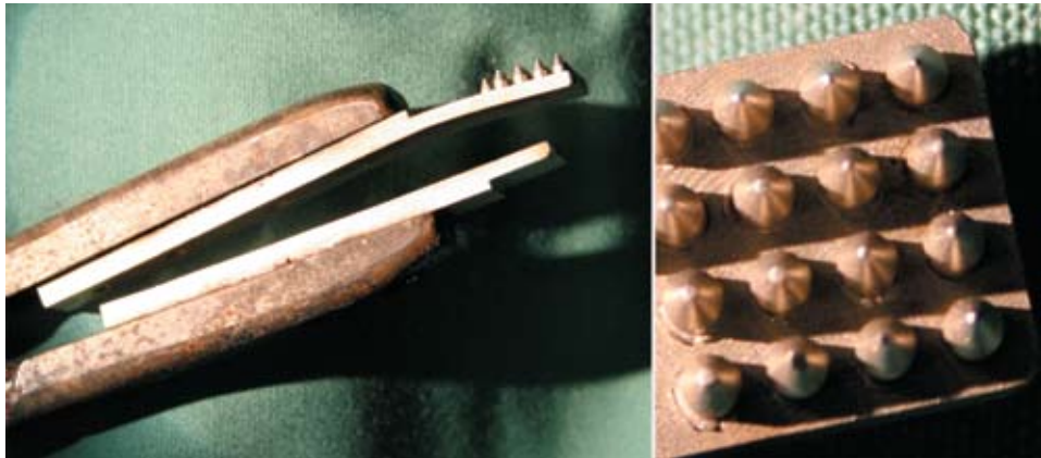
Fig. 2. Photographs of custom-made instrument used for standardized perforation of endplates.
